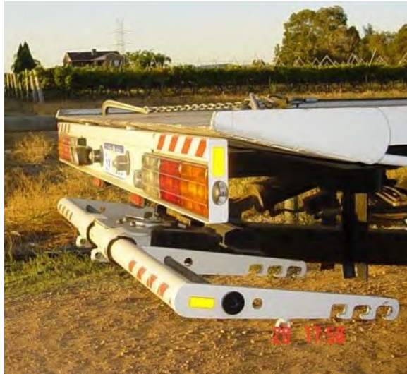
Light bar in normal position
